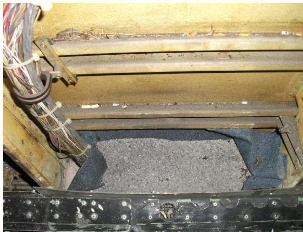
Figure 6: Carpet and sand block airflow from cargo hold to main deck.
