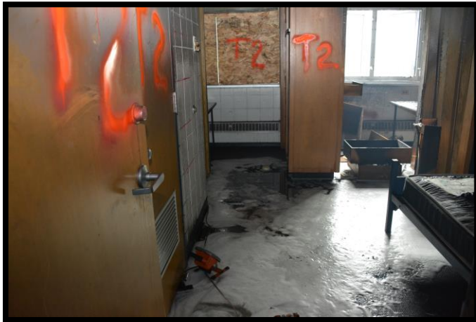
Figure 36-T2 Solid Bore 5.10 second flow 12.8 gallons
