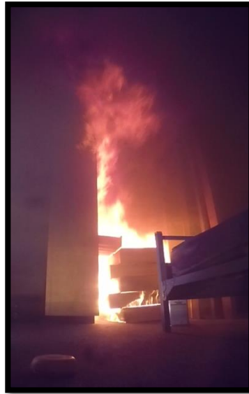
Figure 18-Fire Plume Reaching the Ceiling
