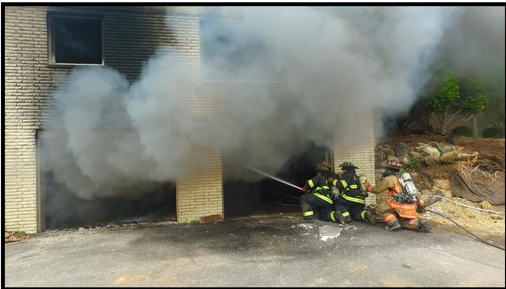
Figure 30-T19 Vehicle Fire in Garage UHP Extinguishment
