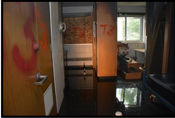
Figure 37-T3 Solid Bore 20.28 second flow 50.7 gallons
