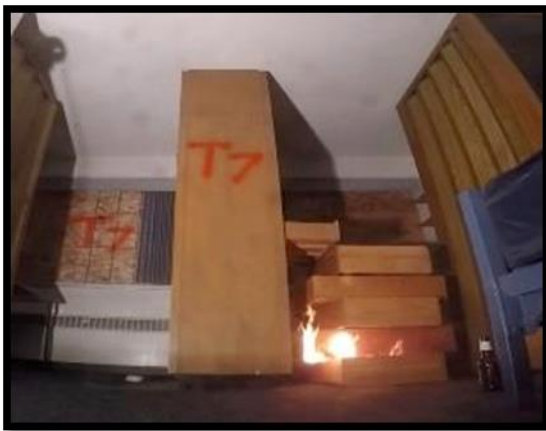
Figure 16-SIP Placed in Bottom Drawer to Initiate the Fires
