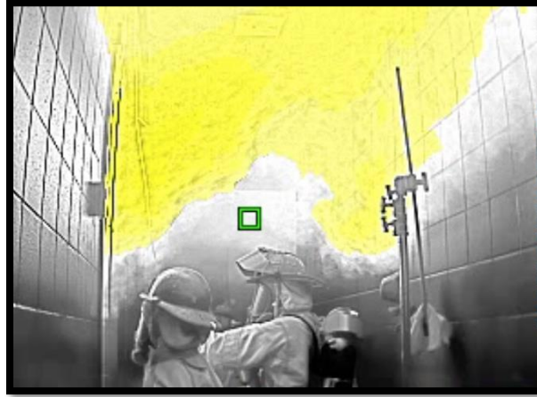
Figure 19-Firefighter Applying Water from the Doorway. Mannequin to the left
